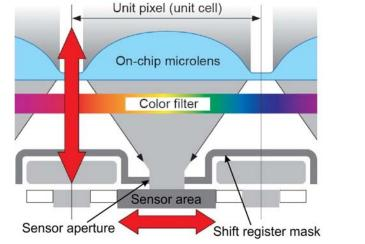
Figure 1 Cross Section of a CCD Pixel (courtesy Sony Corporation)
