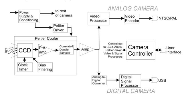
Figure 4 Typical Astro-Video Camera Schematic Diagram
