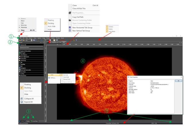
The **MallincamSky Software Window** is segmented into a few regions to make viewing and adjusting the SkyRaider camera easy and intuitive.
