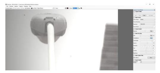
The controls on the right of the screen (**Exposure**, **Gain**, **Gamma**, ...) allow you to change the settings of the SkyRaider.
