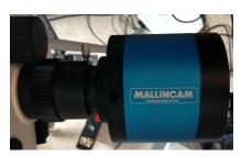
Insert the SkyRaider-DS2.3 Plus (with C-Mount attached) into a 1.25" eyepiece adapter on your Telescope.
