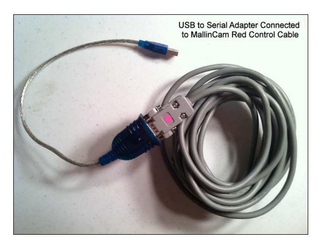
The flat USB end of the combined cable plugs into a USB port on the computer.
