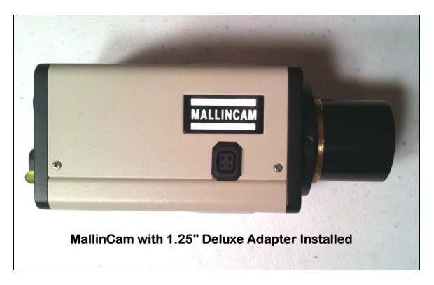
Use the Deluxe Adapter if no focal reduction is desired. The MallinCam will provide a field of view similar to that of a 8mm eyepiece with a 50-degree field of view (FOV). For most telescopes, this results in a fairly high-powered view with a very narrow field of view. To lower the power and increase the FOV, a focal reducer can be substituted for the Deluxe Adapter. The use of focal reducers is not discussed in this document. Other documents are available on this topic.
