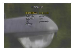
Press the **Down Button** to now select the **SHUTTER** selection (it should say **AUTO**)). Press on the **Right Button** until the choice changes to **MANUAL**. Now press on the **Centre Button** to enter into the Manual **Shutter Sub-Menu**.
