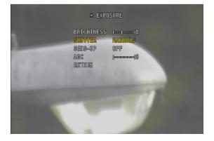
With the **Shutter Sub-Menu** displayed, press the **Left** or **Right Button** to change the shutter time. Notice how the time effects the image. In the image to the right, I have set my Shutter to **1/120**.
