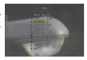
Now press the **Centre Button** on the back of the Mallincam SDI and you will be presented with the **EXPOSURE Sub-Menu**. The **BRIGHTNESS** selection will be highlighted. Using the **Left** or **Right Button** on the back of the camera, experiment with adjusting the brightness of the image.
