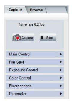
Finally, the Capture Tab has 6 Feature Tab Lines: Main Control, File Save, Exposure Control, Color Control, Fluorescence, and Parameter. Each of these Tabs can be expanded by Left-Clicking on the > symbol.
