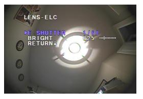
When imaging day time objects, sometimes a bright object may over-power the rest of the image. The All Sky Camera has settings that allow you to help correct or enhance the image from the background.
