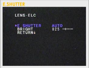
This control allows you to adjust the Electronic shutter and the Brightness of the image.
