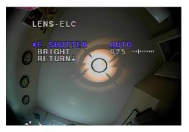
Once finished with adjusting the brightness, it is time to return back to the **Exposure Menu**. Using the **DOWN** button, select the **RETURN** option and press the **CENTRE** button to close the **LENS-ELC** settings Menu (the screen will now return back up to the previous **EXPOSURE** Menu system).
