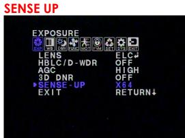
This Setting allows you to adjust the exposure of the All Sky (to a maximum of 8.4 seconds) by utilizing the **HIGH** value of the **AGC** setting and with **E. SHUTTER** set to either **AUTO** or **1/60**. The system will *automatically reduce the shutter speed* whenever light drops below a certain level.
