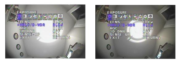
We have experimented with a few different ways to adjust the image on the screen. Now it is time to save the new settings and exit from the On Screen Menu. With the **Main Icons** of the screen push **LEFT** or **RIGHT** on the **Control Button** to select **EXIT** icon. Press **INWARD** on the **Control Button** to display the **EXIT Menu**.
