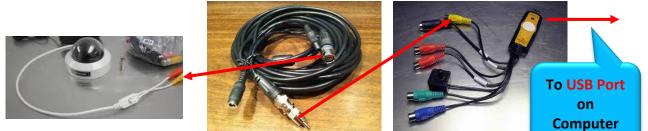
Now all we need to do is start the video display software of your choice to display the image. Remember what ever software choice you made to display the image from the All Sky Camera, it will have an option that allows you to choose the Video Capture Adapter's driver (**x2828** for **MCV**). Once you chosen the driver, you should now see an image of what the All Sky Camera is capturing in the video window of your software.
