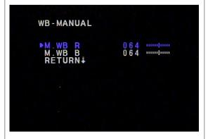
You can set either the **M. WB R** (Manual White Balance Red) or the **M. WB B** (Manual White Balance Blue) settings from a low of **0** to a high of **128**.
