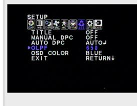
The OSD or On Screen Display that is activated when you press INWARD on the Control Button can be displayed in different colors (Default is Blue).
