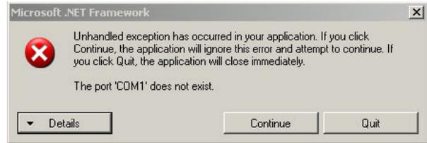
If the ERROR Message box appears, click the "Continue" box and select the "Config" TAB in the MallinCam Control Software.
