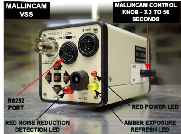
MallinCams with a GREEN power LED have an RS485 computer interface. MallinCams with a RED power LED possess an RS232 computer interface. If your MallinCam possesses either interface, a computer can control it. Proceed to STEP TWO
