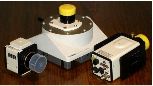
Figure 4. Author's Astro-Video Cameras: The author owns three cameras for video astronomy (from left): Mallincam Junior, Toshiba IK-WB11A net-cam, and Mallincam Xtreme. (images by author)
