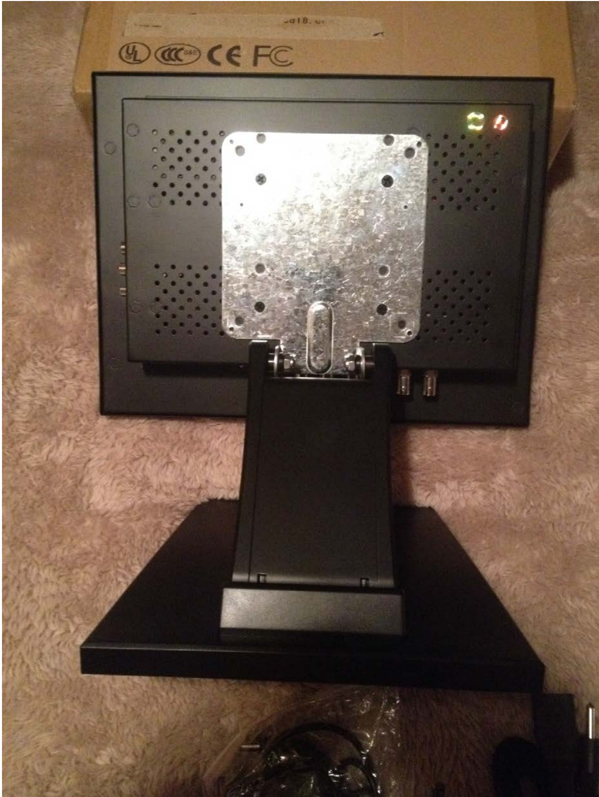
This shows the metal plated screwed to the back of the monitor.
