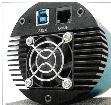
This close-up view of the camera's back panel shows the cooling fan and cable connections.
