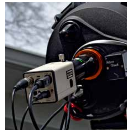
For faint objects, the authors hooked up the MallinCam Jr PRO to their 8-inch Celestron EdgeHD Schmidt-Cassegrain telescope.
